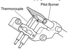
Figure 26 - Correct Pilot Flame Pattern
